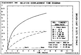
CLAY .- Atlas pile; EXAMPLE 2: tested Atlas Palen. Koekelare. Belgium. at Approximate pile length is 13 m. with an estimated pile diameter of 0.51 m. ond tip diameter of 0.61 m. The founding stratum is generally clay. This is perhaps, one of the more complex pile types to analyse: however it displays the characteristic behaviour in time.
