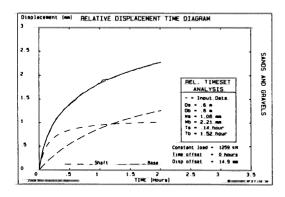
In these examples of pile behaviour the and base are appropriately distinguished by the separate individual hyperbolic functions, regardless of the taken and events before the load has achieve its constant value. When these functions are added together on the vertical scale they can be made replicate the measured behaviour.
